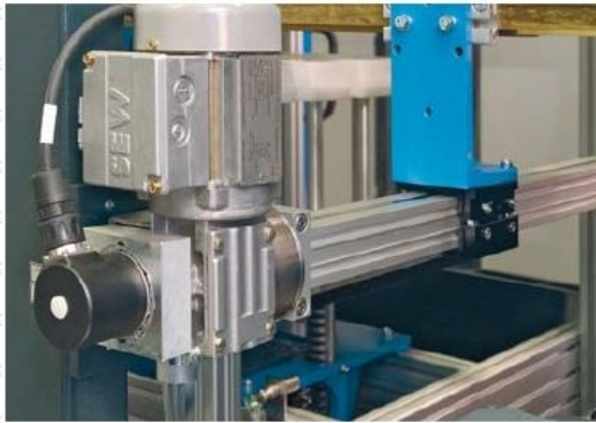
Separately actuated width-adjustment mechanisms for the chain guides
