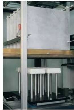
Flexible stacking station for rigid or movable shaft configuration
