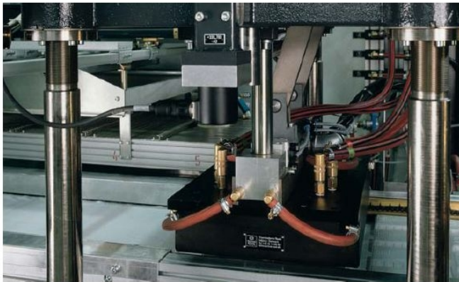
The top table in the forming station is actuated by servomotors to ensure precise table movements and maximum repetitive accuracy
